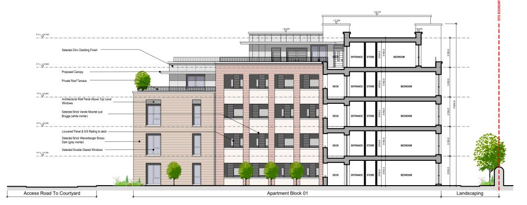
Apartment Block 01 - South West Sectional Elevation Scale 1:200
